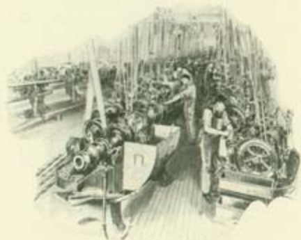
Long rows of "automatics" turn out thousands of cups, cones and rollers "in the green" each day
