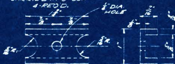
VALVE LIFTER HOUSING BRACKET 4-REQ'D. MATERIAL - STEEL
