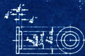
VALVE SPRING RETAINING WASHER MATERIAL - BRASS 8-REQ'D.
