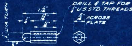
ADJUSTING NUT MATERIAL - \frac{5}{16} " STEEL HEX BAR 8-REQ'D.
