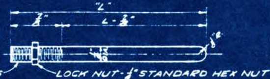
INTAKE VALVE PUSH ROD 4-REQ'D. 'L' = 3" EXHAUST VALVE PUSH ROD 4-REQ'D. 'L' = 3" MATERIAL - \frac{1}{4} " STEEL DRILL ROD
