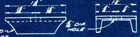
EXHAUST MANIFOLD CLAMP 2-REQ'D. MATERIAL ~ 1 \frac{1}{2} " x \frac{1}{2} " x \frac{1}{2} " LG. CHANNEL
