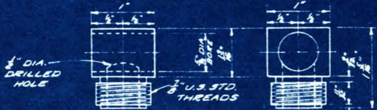
THROTTLE TEE 1-REQ'D. MATERIAL - STEEL
