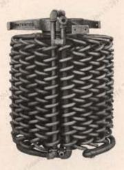
Generator Heart of Steamer a boiler large enough to supply the necessary power to propel it at a good speed up all grades and over the poorest roads it has been poorly constructed and a generator of greater horse power should be put in. Upon the generating outfit depends the pleasure of operating a steam automobile.
