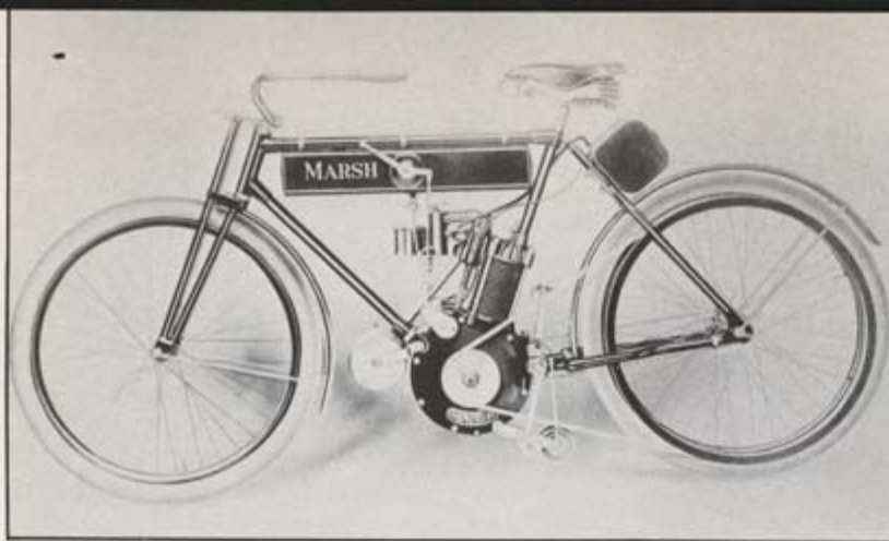
1903 Marsh motorcycle. Motor integrated into frame. High ratio belt drive.
