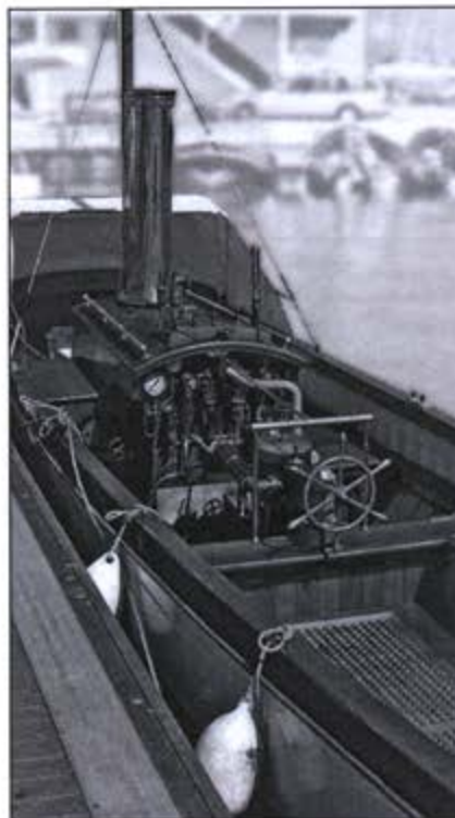
Kariat steam launch moored at Cowes. Once the only surviving LIFU vessel with original engine. Length 35 ft. Beam 6 ft. 9 ins, Engine 35 shp. Boiler pressure 200 lbs. Speed about 12 knots.
