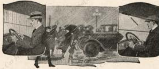
Eveready automatic windshield cleaner which uses the vacuum in the intake to operate a wiper arm.
