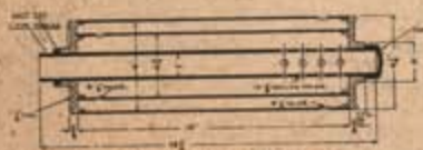
Sectional view of the muffler showing the internal structure.
