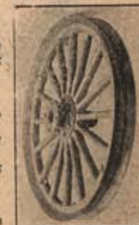
DYKE REAR WHEEL, Showing Flange with Rim attached.
