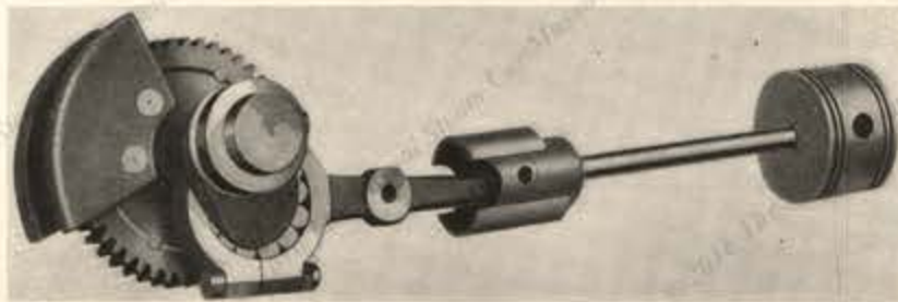
Assembly of piston, crosshead, connecting rod with roller bearing at big end, and crank shaft showing counter-weights
