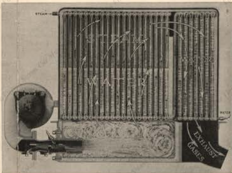
Doble-Detroit Steam Generator—Sectional view. Large arrows indicate flow of gases of combustion—small arrows indicate flow of water. Water enters the lower headers of the Economizer Sections, shown at the right. Steam leaves the upper headers of the Evaporating Sections, all those above the combustion chamber
