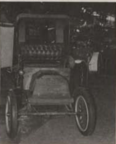
"The hood was modified to look like the hood over a gas-engined car, although the engine and water tanks are under the seat and rear compartment."
