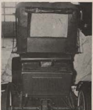
"The large water tank holds 30 to 35 gallons; the tank is not under pressure, can be refilled at any time without the least danger."
