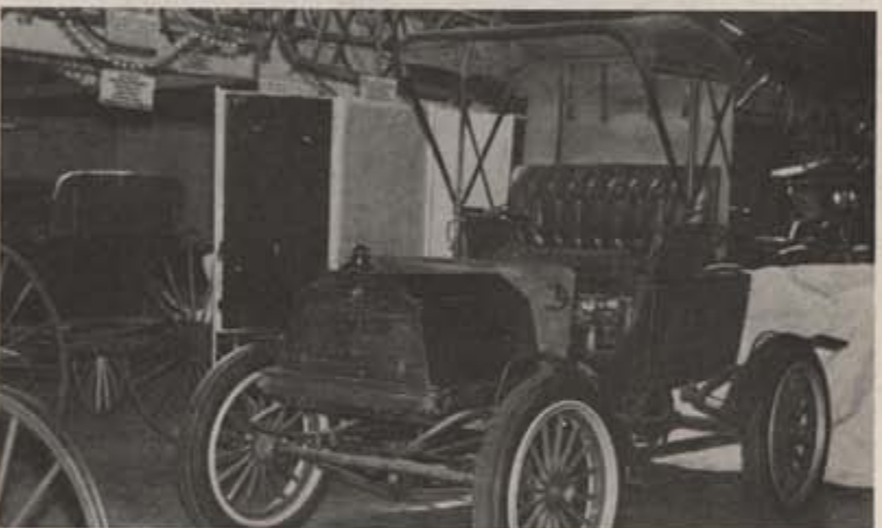
"In the front part of the body is the 15-gallon fuel tank, steam and air gauges, and the tool box, necessary to carry an ample supply of tools."
